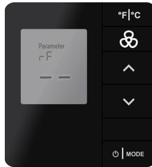
Figure 10: Setup RF Channel
